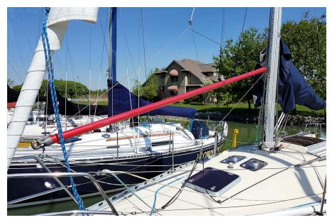
that hauling in on the downhaul had always been difficult in a strong wind. I dead-ended the downhaul at the deck and attached a block-and-tackle combination to the pole to give the crew a 2:1 mechanical advantage.
