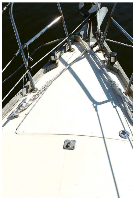
Nurdle's foredeck-mounted sidelights were underfoot and prone to damage, above. John replaced them with a combination lantern protected by the pulpit, at right.
