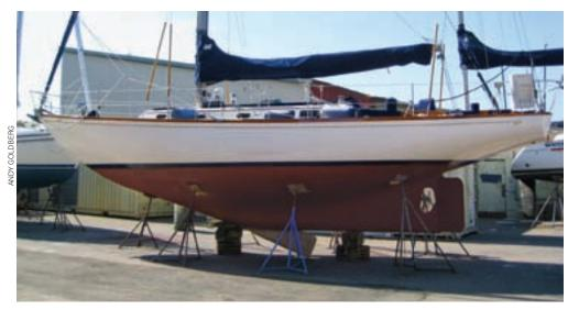
modified-full type with the leading edge of the keel pretty well defined from the forefoot. The rudder is on the trailing edge of the keel on a highly raked rudder stock. On many of his early designs, Tripp used barn-door-style rectangular rudders mounted on vertical stocks. That can't be a fast shape but it sure looks right and totally Trippy.
