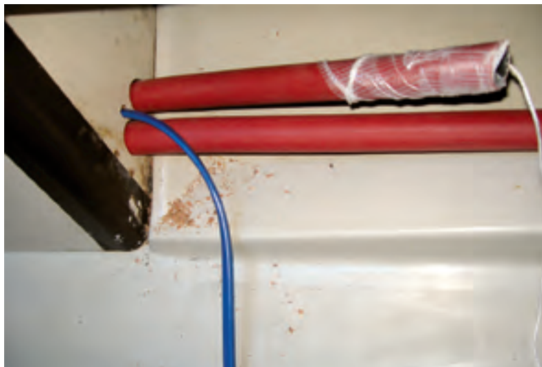
The hot-water tank is in the cockpit locker and Graham put a step over it to protect it, at left. The gray tank is the expansion tank. Running 50 feet of heater hose through the boat, above, was labor intensive but worth it.
