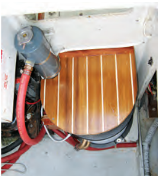
The hot-water tank is in the cockpit locker and Graham put a step over it to protect it, at left. The gray tank is the expansion tank. Running 50 feet of heater hose through the boat, above, was labor intensive but worth it.
