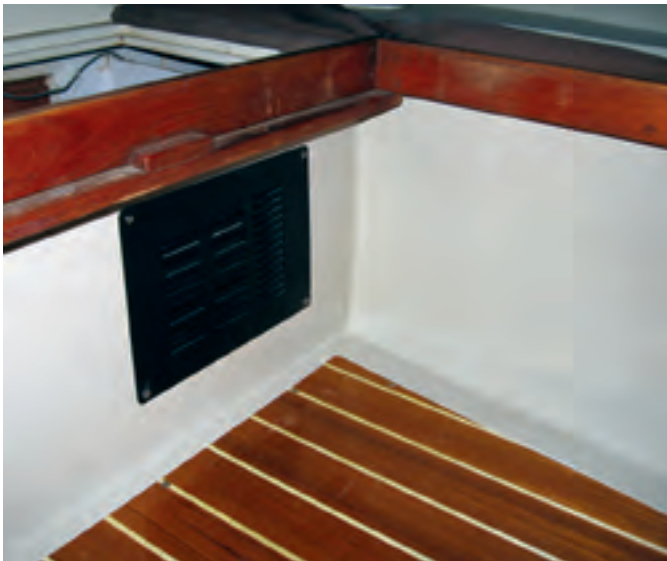
The larger radiator warms the saloon, at left. It's under the aft leg of the U-shaped settee and draws air from the galley. The Espar heater, above, is installed aft under the cockpit. It draws combustion air from the cockpit locker and the exhaust exit is in the transom.
