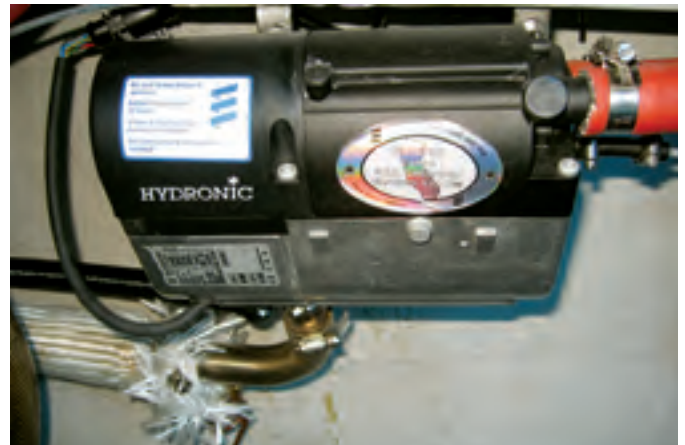
The larger radiator warms the saloon, at left. It's under the aft leg of the U-shaped settee and draws air from the galley. The Espar heater, above, is installed aft under the cockpit. It draws combustion air from the cockpit locker and the exhaust exit is in the transom.
