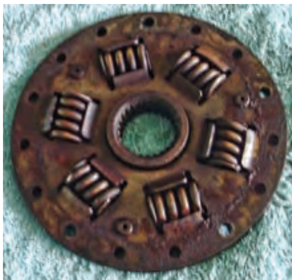
The old damper plate doesn't look too bad but one of the clips was off and the springs were loose.
