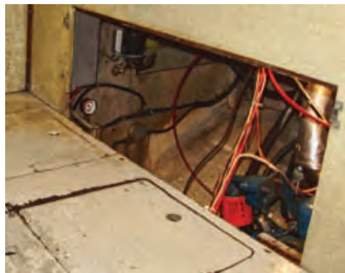
On Bob's boat, the rear engine mounts are attached to the transmission case by L-brackets, at left. The two top nuts holding the transmission to the bell housing are visible beneath the yellow oil filter. Bob's primary work area was through an access panel in the rear quarter berth, at right. That put him at the back of the engine and above the transmission.
