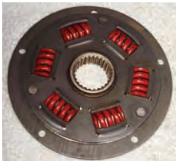
The damper plate is constructed of two plates and springs. The transmission shaft fits into a toothed hole in the center.
