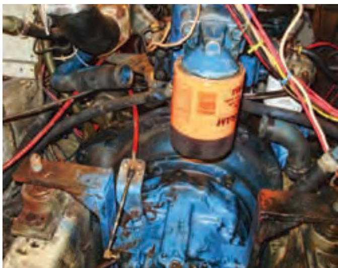
On Bob's boat, the rear engine mounts are attached to the transmission case by L-brackets, at left. The two top nuts holding the transmission to the bell housing are visible beneath the yellow oil filter. Bob's primary work area was through an access panel in the rear quarter berth, at right. That put him at the back of the engine and above the transmission.
