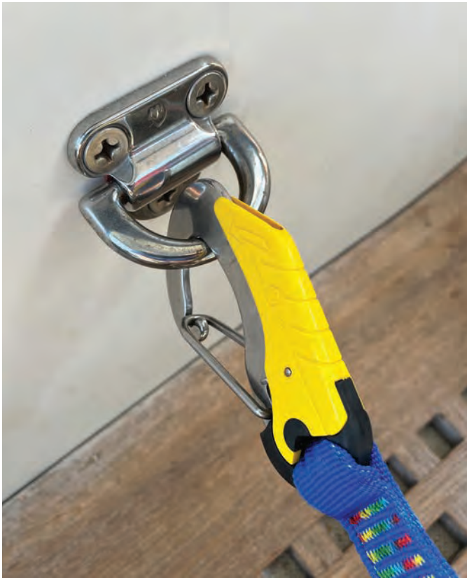
These large cockpit pad-eyes allow the tether to move with the user.
