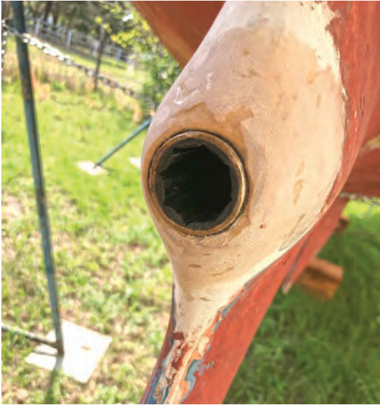
The epoxy is smoothed out and hardened, with the shaft removed.
