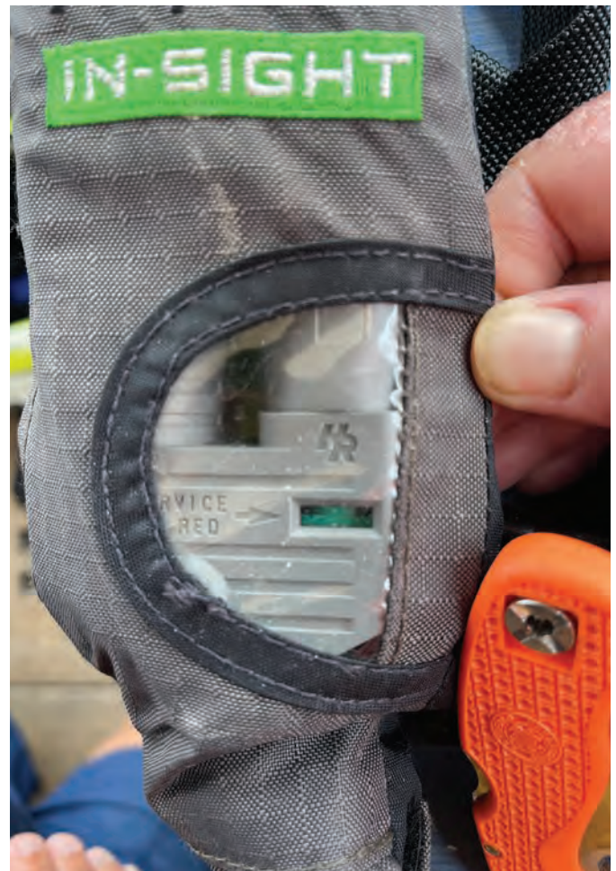
The vest the author was wearing when he went overboard shows the inflator mechanism armed and ready, post submersion.
