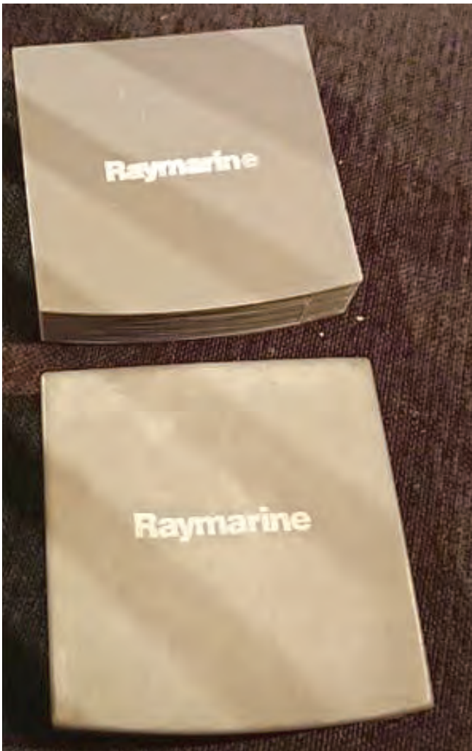
Raymarine covers: The top one is the new 3D printed version. Photo credit JP Nurro.
