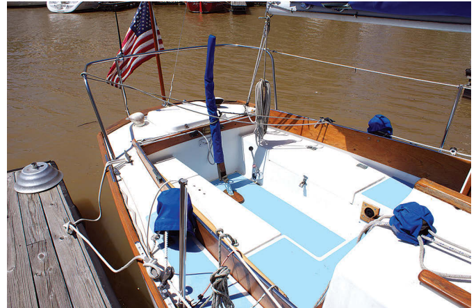
No serious provision is made on the foredeck for anchoring, at left, but the cleats and fairleads are adequate. The blue non-skid has held up fairly well on Scotch's Too III . The toerail and rubbing strake are attractive and useful. Teak cockpit coamings, at right, are indicative of the quality of materials Cape Dory Yachts employed. There's good stowage beneath the seats, which are long enough to lie down on.
