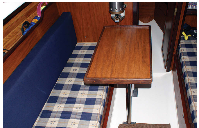
The galley is partially under the bridge deck and spans the cabin, at left, and the electrical panel and basic electronics fit tidily on the bulkhead. On Scotch's Too III , the table fits on stainless-steel posts, either close over the port settee, at right, or centered between both.
