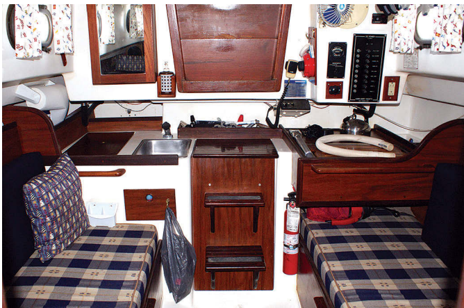
The galley is partially under the bridge deck and spans the cabin, at left, and the electrical panel and basic electronics fit tidily on the bulkhead. On Scotch's Too III , the table fits on stainless-steel posts, either close over the port settee, at right, or centered between both.
