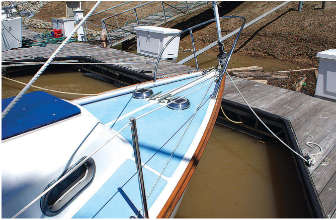
No serious provision is made on the foredeck for anchoring, at left, but the cleats and fairleads are adequate. The blue non-skid has held up fairly well on Scotch's Too III . The toerail and rubbing strake are attractive and useful. Teak cockpit coamings, at right, are indicative of the quality of materials Cape Dory Yachts employed. There's good stowage beneath the seats, which are long enough to lie down on.
