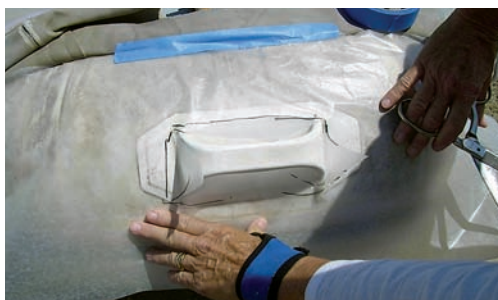
With rough cutouts made to fit around handles and other fittings, the pattern can be fitted on the dinghy.
