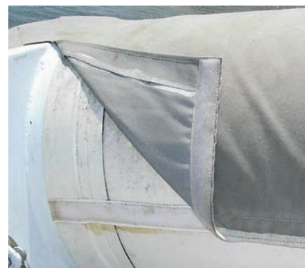
After the pattern has been transferred to the fabric, at left, the cut edges can be painted with Liquid Rope Whipping to protect them. It takes two coats to look nice and last well. After more than three years of use, the cutout for the handle on the bow of the dinghy still looks tidy, center. The loop Velcro is sewn directly to the fabric cover, while the hook side is first sewn to vinyl and then glued to the dinghy, at right.
