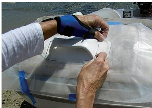
Since the cut edges will not be exact or smooth, extra pieces of plastic are taped as necessary to fine-tune the fit.
