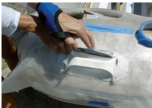
Once the pattern has been shaped to the dinghy, the rough cutouts must be smoothed and the extra pieces cut away.
