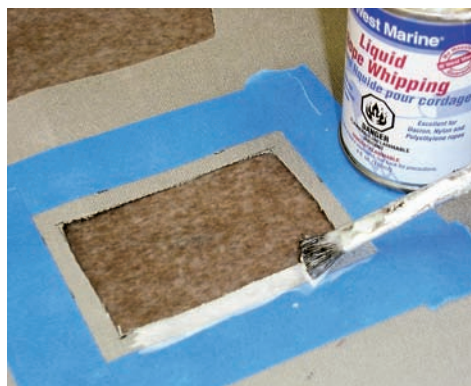
After the pattern has been transferred to the fabric, at left, the cut edges can be painted with Liquid Rope Whipping to protect them. It takes two coats to look nice and last well. After more than three years of use, the cutout for the handle on the bow of the dinghy still looks tidy, center. The loop Velcro is sewn directly to the fabric cover, while the hook side is first sewn to vinyl and then glued to the dinghy, at right.
