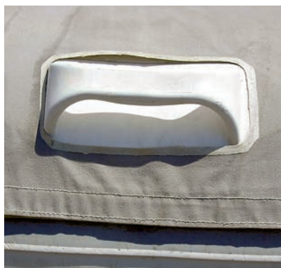
After the pattern has been transferred to the fabric, at left, the cut edges can be painted with Liquid Rope Whipping to protect them. It takes two coats to look nice and last well. After more than three years of use, the cutout for the handle on the bow of the dinghy still looks tidy, center. The loop Velcro is sewn directly to the fabric cover, while the hook side is first sewn to vinyl and then glued to the dinghy, at right.
