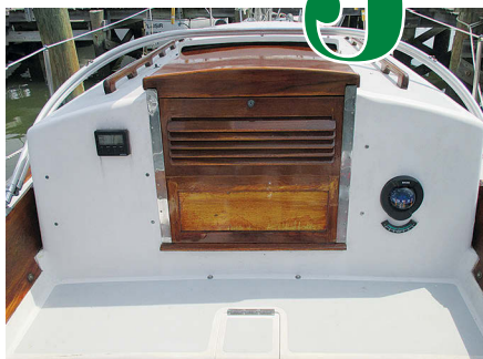
The depth sounder and compass are mounted on the cockpit bulkhead, above. The VHF is down below. John uses a hand-held GPS. Another compass fits on centerline in a bracket installed in the bridge deck.
