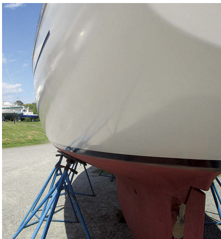
The original 1967 white topsides gelcoat is hand buffed and still shines, above, even if it is no longer a mirror finish.
