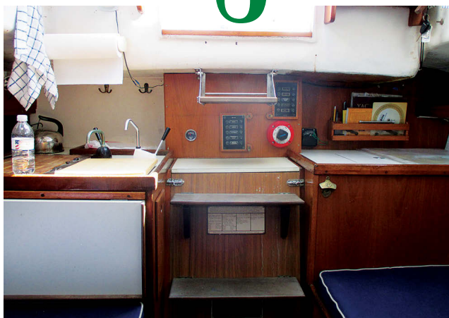
The galley is split aft with the icebox under a chart table. John modified the original icebox to add the chart table. The two-burner Origo stove is outboard of the sink on the starboard side.
