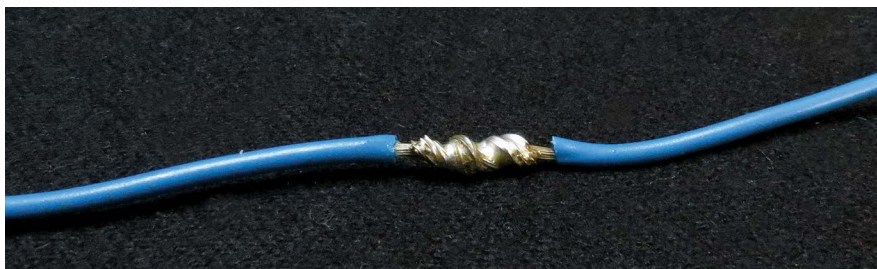
A good solder joint has a smooth surface that closely follows the contours of the wires.
