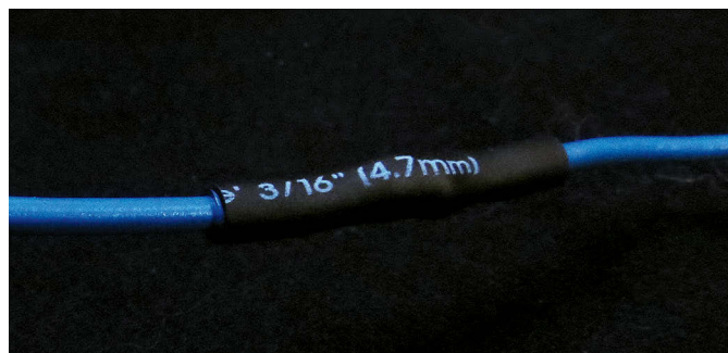
To ensure a waterproof seal on the insulation, the heat-shrink tubing should extend at least ¼ inch either side of the bare wires.
