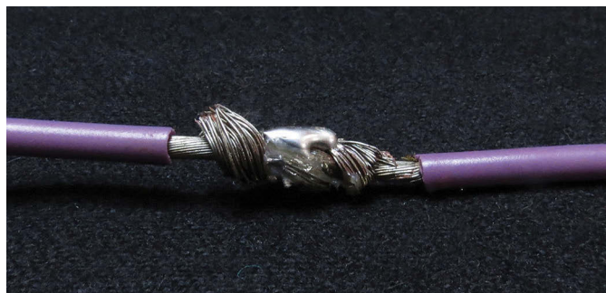
A joint with too much solder looks bulky, above. If the joint has too little solder, the strands of the wire are clearly visible, above right. Both joints need to be redone.
