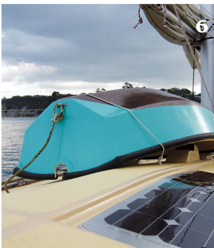
Being able to easily pull her dinghy on board is important to Annie. The first step is to drop the lifelines (1). She then hauls the boat over the rail (2). Once the balance point is inboard, she turns the dinghy around on the deck (3). Because it's so light, she can then flip it over (4) and maneuver it into position (5), where she lashes it securely (6).
