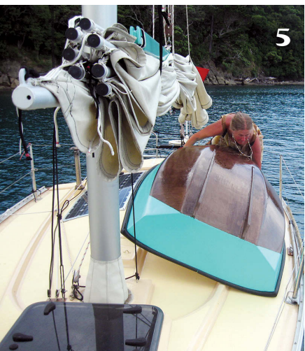
Being able to easily pull her dinghy on board is important to Annie. The first step is to drop the lifelines (1). She then hauls the boat over the rail (2). Once the balance point is inboard, she turns the dinghy around on the deck (3). Because it's so light, she can then flip it over (4) and maneuver it into position (5), where she lashes it securely (6).
