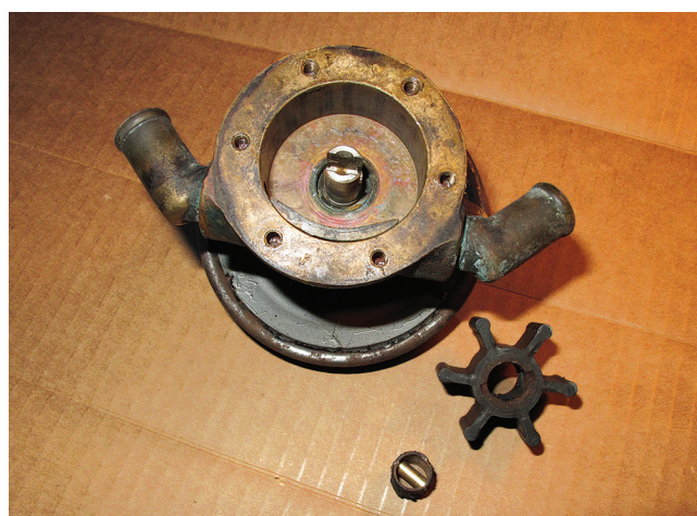
Ellen expresses glee and relief at Entr'acte's arrival in Paris, at top. On the way, the engine had overheated frequently due to a damaged impeller in the raw-water pump, above. The center hub, which held the pin that engaged the drive shaft, broke loose — but gradually.
