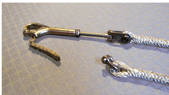
The lifeline gate has a threaded toggle to fit the pelican hook on one end and a shackle on the other.
