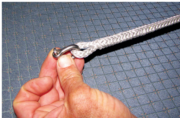
It's important to allow about two inches extra length for the bunching at the eye-splice where the rope has to expand to cover the inserted tail.
