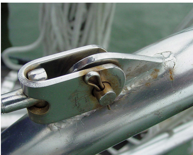
A stress crack and some corrosion are visible at the base of the lifeline-attachment eye where it's welded to the pulpit, at left. Also, the cotter pin looks loose and could fall out if the clevis pin it's securing rotates over time due to vibration. Where a vinyl-coated lifeline passes through a stanchion, the coating can chafe away, at right, creating a path for water to enter the wire and initiate corrosion.
