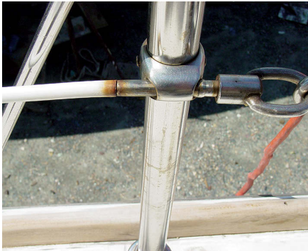
Even when a vinyl coating is undamaged, water can wick between it and the terminal fitting and penetrate the wire, at left. A vinyl coating can crack due to age, especially at a stress point, such as this stanchion, at center, allowing moisture to enter and corrosion to begin. The “running rust” stain extending from beneath this stanchion base, at right is a sure sign the mounting hardware (or the stanchion itself) is corroding. It might also indicate that water has penetrated the deck laminate. The stress cracks in the gelcoat are another sign of trouble.
