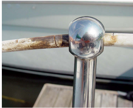
Even when a vinyl coating is undamaged, water can wick between it and the terminal fitting and penetrate the wire, at left. A vinyl coating can crack due to age, especially at a stress point, such as this stanchion, at center, allowing moisture to enter and corrosion to begin. The “running rust” stain extending from beneath this stanchion base, at right is a sure sign the mounting hardware (or the stanchion itself) is corroding. It might also indicate that water has penetrated the deck laminate. The stress cracks in the gelcoat are another sign of trouble.
