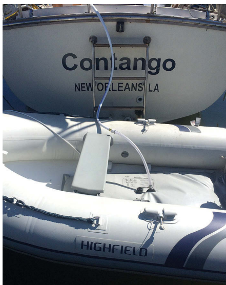
With the dinghy tied to the boat's stern, a garden hose connects the bladder to the 12-volt pump (not pictured) that transfers the water into the ship's water tanks.
