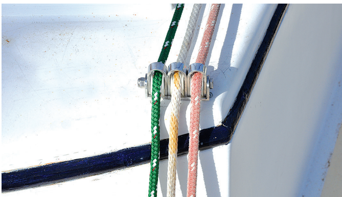
A three-sheave block carries the jib furling line, the staysail furling line, and the staysail outhaul over the top of the forward coachroof, at left. A single-sheave block, at right, routes the jib furling line to the deck. This is a one-off made in a slightly different way from the other blocks.
